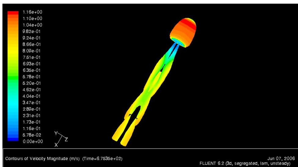
Figure 4: Contours of velocity magnitude at Re = 300 plotted on iso-contours of the second invariant of the deformation tensor
